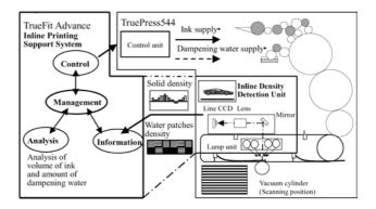
Figure 2. The Inline Printing Support System(TrueFit Advance)
